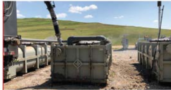
Used FerroSorp being vacuumed out
