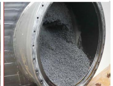
Spent FerroSorp can be vacuumed out of vessel
