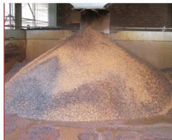
Used FerroSorp free flowing during change out
